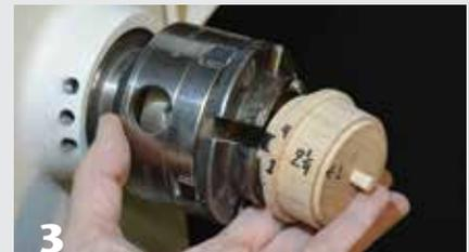
Use a straightedge to ensure a flat end surface. Drill a hole and glue in a dowel. Mark the location of the faceplate in the chuck so it can be remounted later in exactly the same position.
