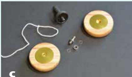
A hub-style kit requires a larger diameter hole to accept the hub, which is then mounted on a small screw chuck.
