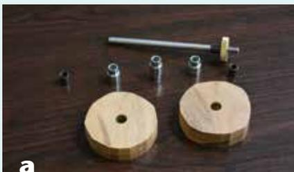
Similar to a pen kit, this style of yo-yo kit makes use of brass tubes glued into the blank, a mandrel, and bushings.
