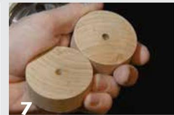
Turn a cylinder of a consistently dense hardwood. Drill for the axle, turn to final diameter, and part off. These are your yo-yo blanks ready to mount and turn.
