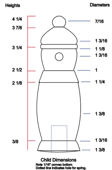
Figures 2–4. The basic measurements for turning a family of penguins.
