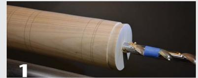
Mark the blank with key diameters and drill a hole in the bottom end for the animating spring.
