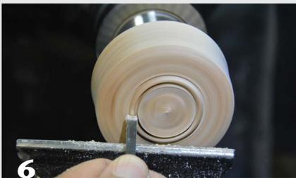
Mount the wheel blank on a screw chuck to turn it to size and shape the outside.
