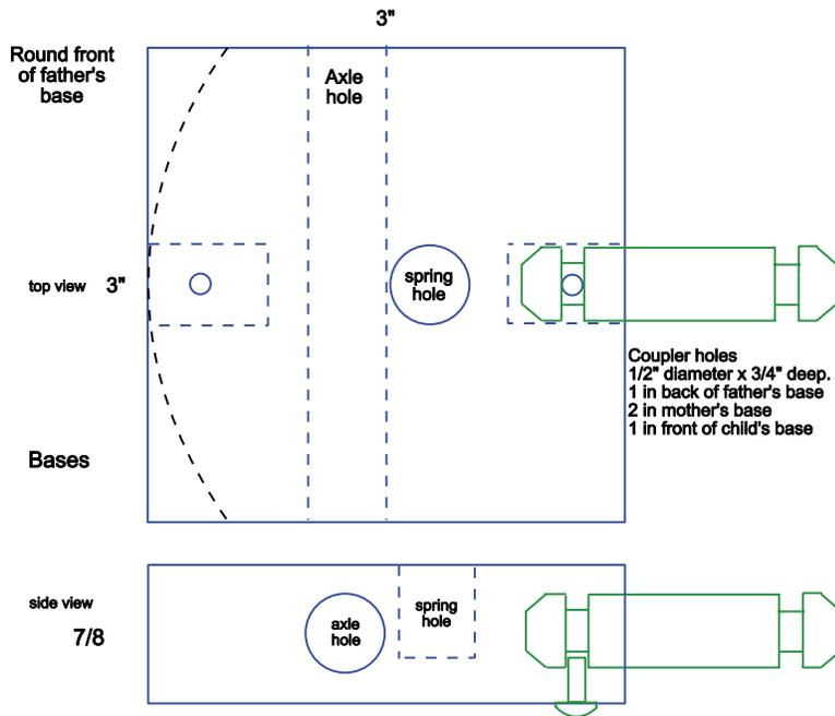
Figure 1. The plan for the penguin bases.
