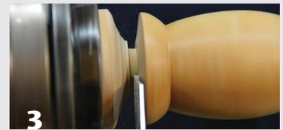
When parting off the figure, make the base slightly convex, or dome-shaped. The bottom need not be flat since the penguin will be mounted on a spring.
