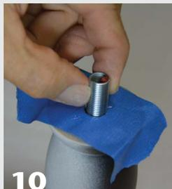
Mask off the base of a penguin and attach the spring with epoxy.
