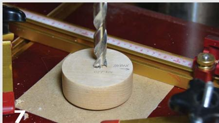
Plug the screw-chuck hole with a dowel and drill the axle hole off center.
