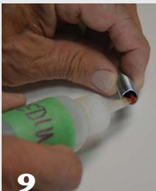
Attach a restraining cord inside the springs with a dab of cyanoacrylate glue.
