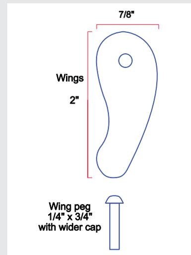
Figure 6. Shape the wings from thin hardwood stock and turn small pegs to hold them in place.
