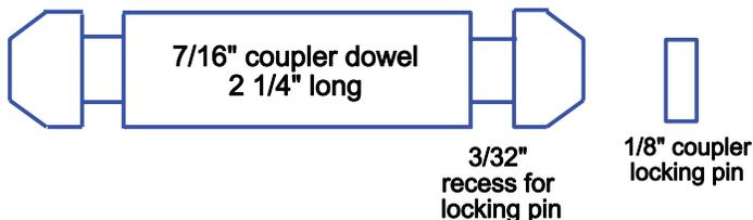
Figure 5. Two wooden couplers connect the three bases, and the locking pins hold the couplers in place.
