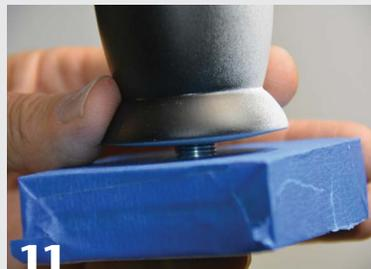
When attaching the spring to the base, leave a  $\frac{1}{8}$ " gap so the bird can wobble.
