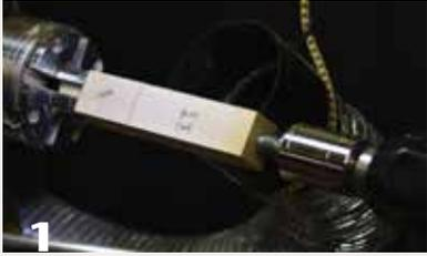
1 Mark the head/body blank, delineating each section. Begin by turning only the body; leave the head section square. Drill holes for the neck and feet, as shown in *Figure 1*.
