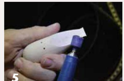
5 A rotary tool with a small drum sander makes quick work of final shaping and sanding the bird's body.
