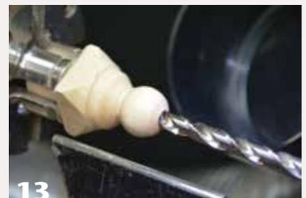
11 Remount the unturned head blank. Turn most of a sphere, but leave some supporting wood for drilling. First drill a larger hole for the beak, then a smaller hole within the first for reverse-mounting on a screw chuck to finish turning the back of the head.
