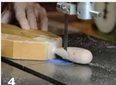
4 Mark and cut away the underside of the bird's body. Note the still-square head section is held securely in a wooden handscrew clamp for safe bandsawing.
